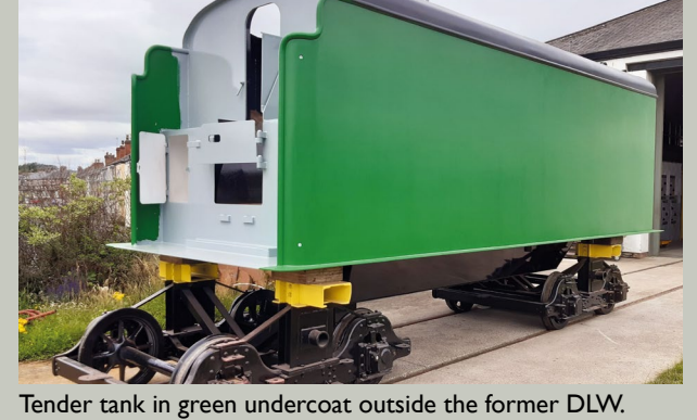
Tender tank in green undercoat outside the former DLW.
