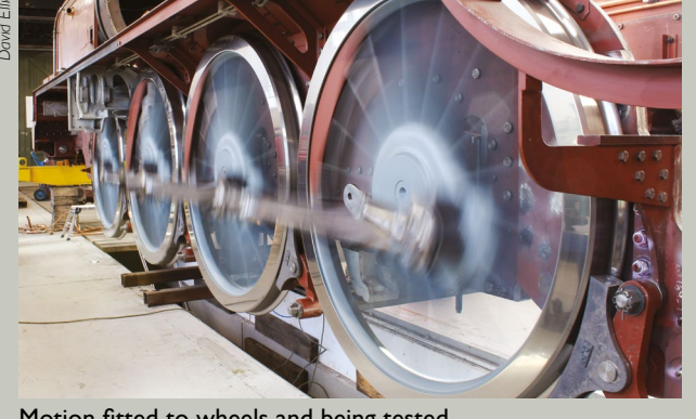
Motion fitted to wheels and being tested.
