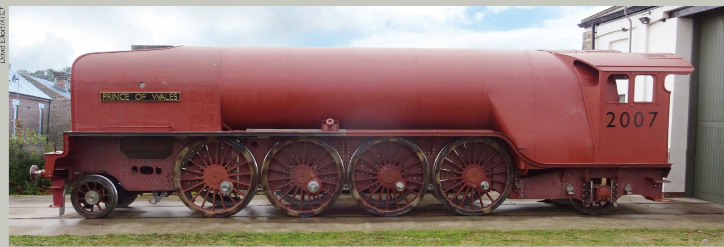
No. 2007 Prince of Wales outside the former Darlington Locomotive Works, with boiler cladding demonstrating what the engine will look like as progress is made.
