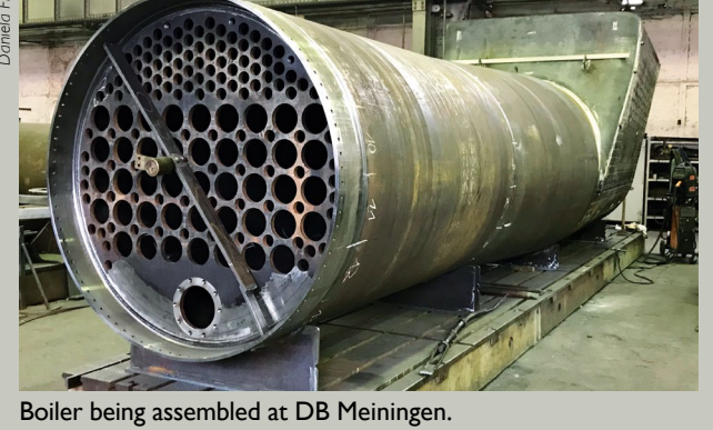
Boiler being assembled at DB Meiningen.
