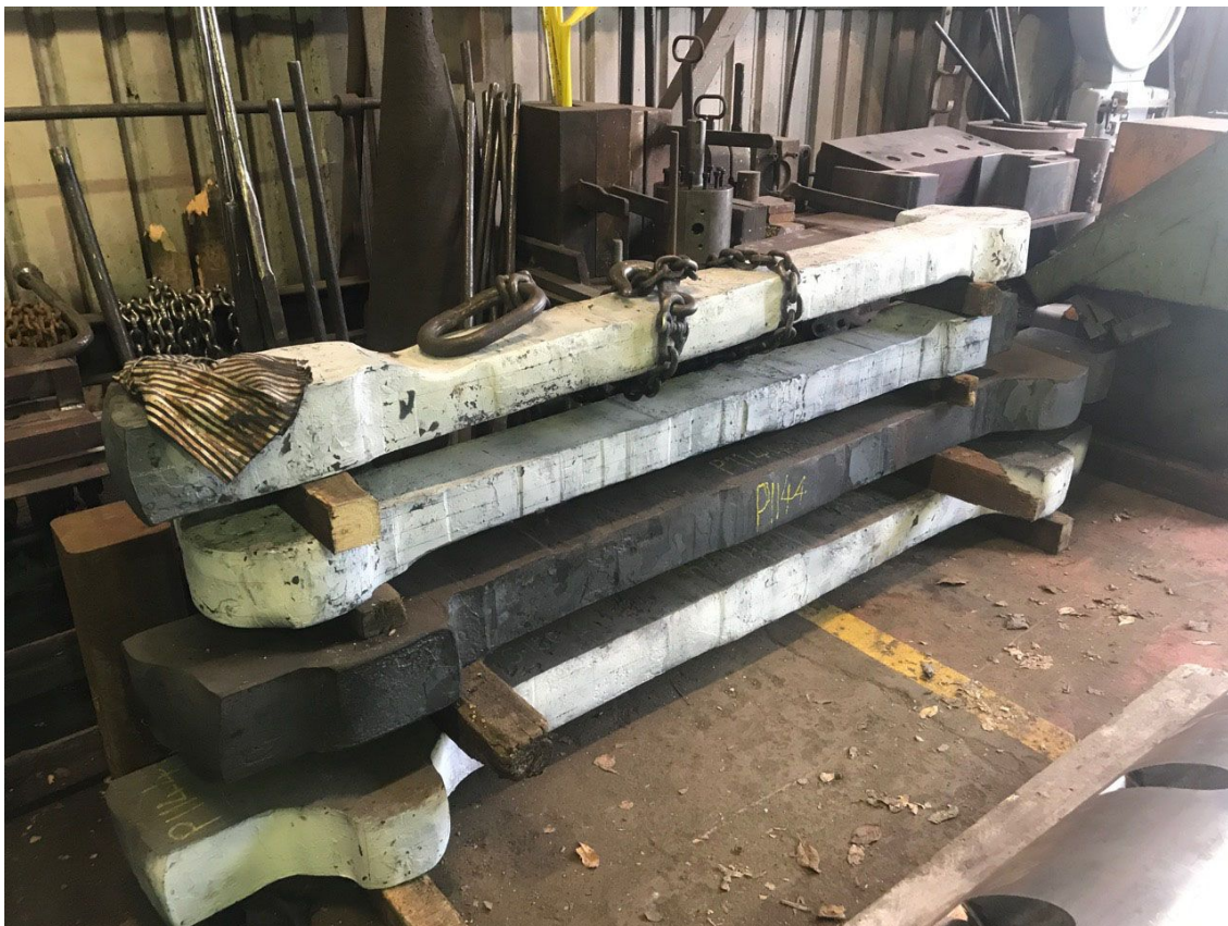
Four forged coupling rods at Stephenson (Engineering) Ltd - Robert Stephenson/A1SLT
