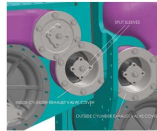
**3D CAD of the cylinder block showing valve covers and split sleeves.**
