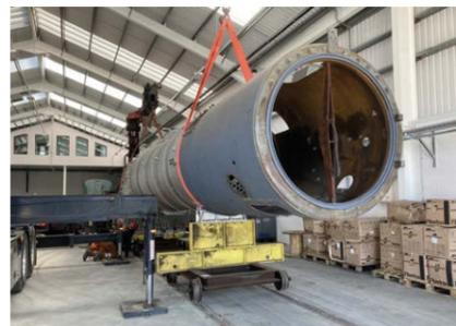
Above and right: With the tender tank moved, *Tornado's* boiler was extracted from the old works, trundled through Darlington and off-loaded at DLW2.
