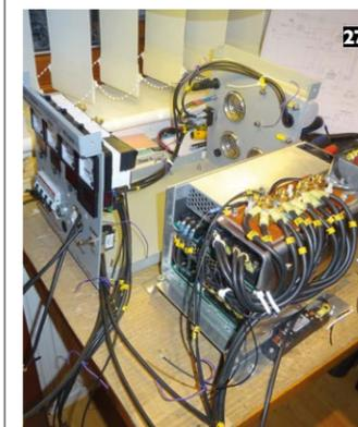
28. Fully assembled Shore Power Supply electronics.
