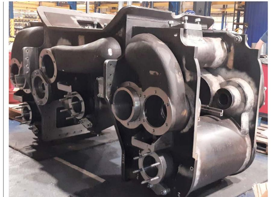
**Trial fitting covers and blanks to rear of cylinder block.**
