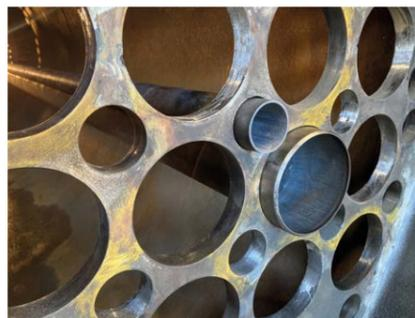
**Trial fitting small and flue tubes.**
