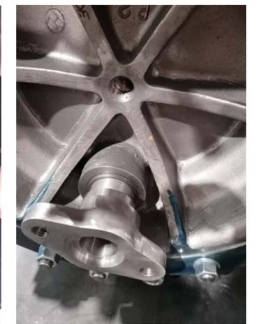
**Centre right: A BR pattern cylinder relief valve fitted.**
