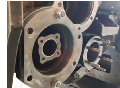
**Rear inside exhaust valve cover assembly trial fit.**
