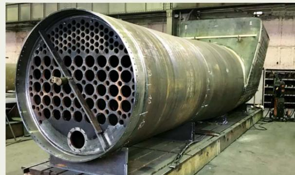
First new boiler being assembled at DBM.
