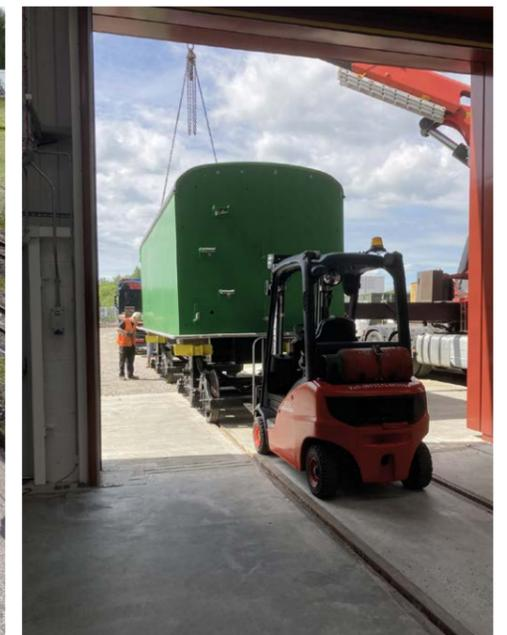
The tender tank and accommodation bogies were then unloaded at DLW2.
