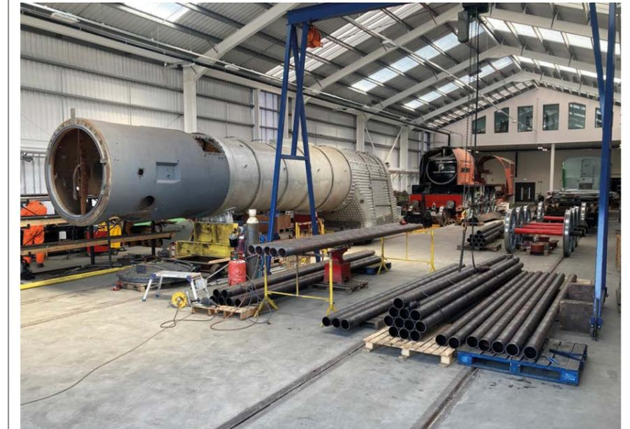
**Flue tubes and boiler in the new works.**
