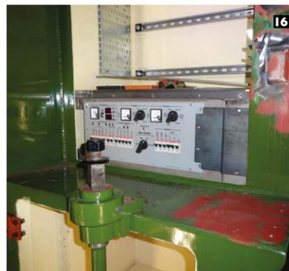
17. ETCS I/O Panel in its test location on the front of the tender and operating on shore power.
