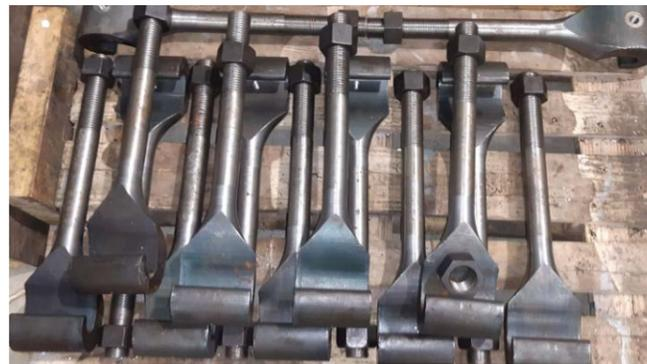
**Compound curvature CNC machined on tender spring hooks.**
