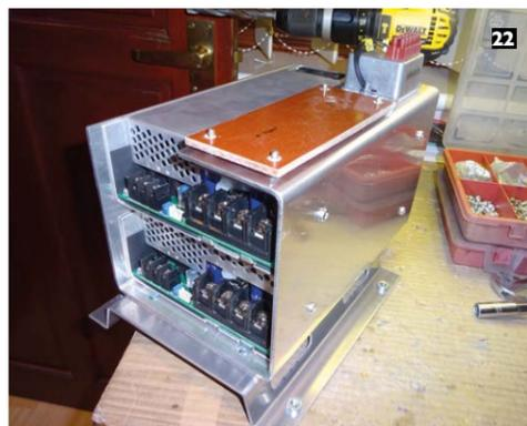
23. Chassis with output busbars in place.
