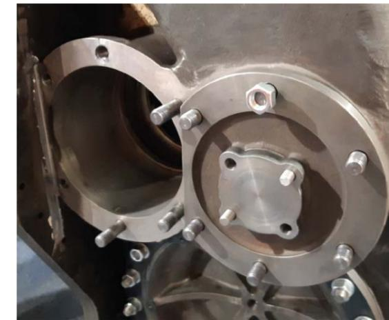
**Centre left: Front left-hand inlet valve trial fit.**
