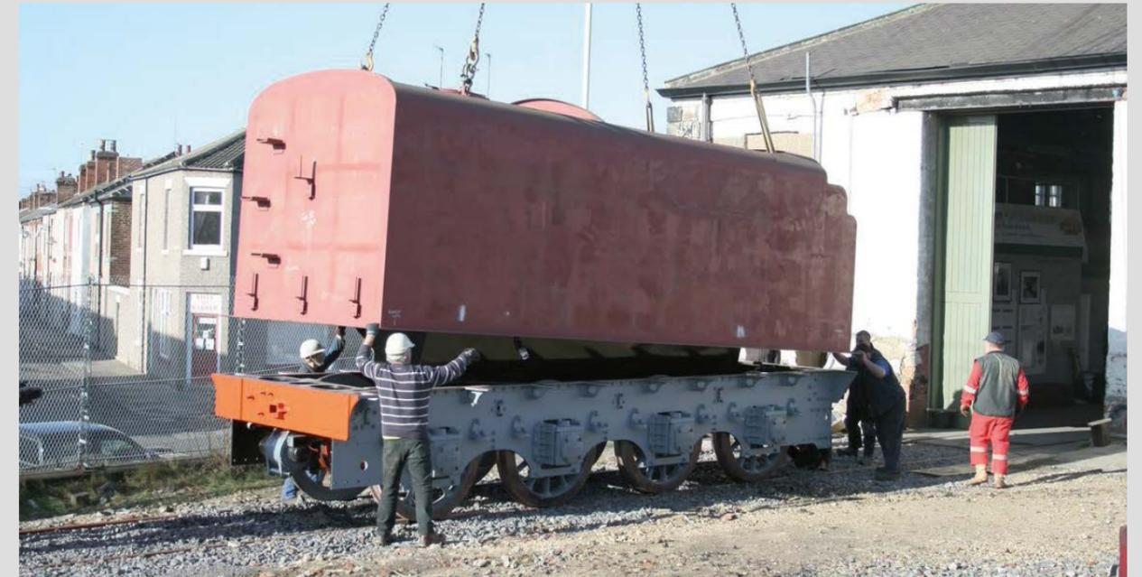
Fifteen years ago we were also moving tender tanks around the yard at DLW1. This is *Tornado's* being fitted to its frames.
