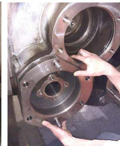
**Centre middle: Offering up rear inside exhaust valve cover assembly.**
