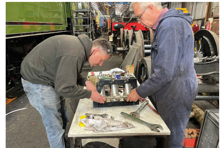
David Wright and Andy Morgan from LMS work to reassemble the brake equipment.
