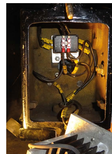
Above left: New flexible conduit and connector for the lower front marker, also showing the front buffer beam umbilical cable and connector.
