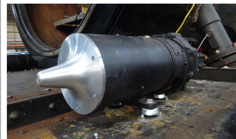
Above images : New turbogen mounted on the driver's side front running plate.
