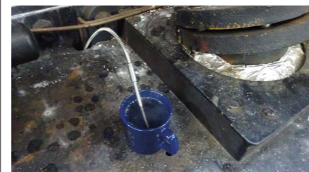
Steam chest temperature gauge probe in hot water.
