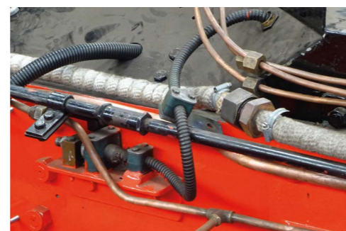
Right below: Atomiser steam pressure switch on the inside frame under the smokebox (to be renewed). TCC
