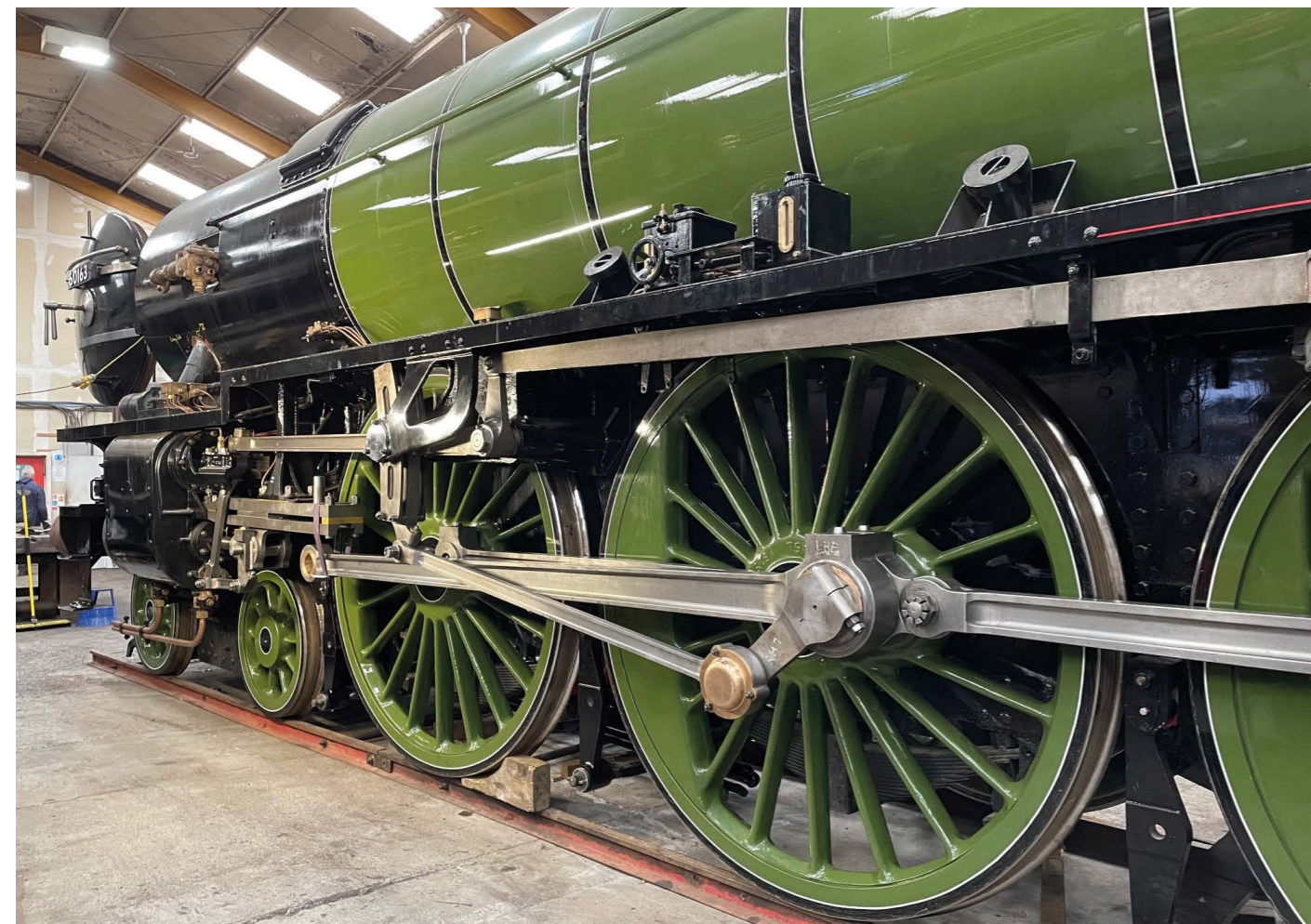
Above: The rest of the motion back in place, just awaiting connecting to the crosshead.
