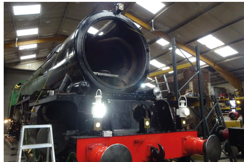
Testing the front head and marker lamps.
