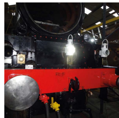
Testing the front centre headlamp.
