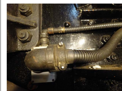
Above left: New flexible conduit and connector for the lower front marker, also showing the front buffer beam umbilical cable and connector.
