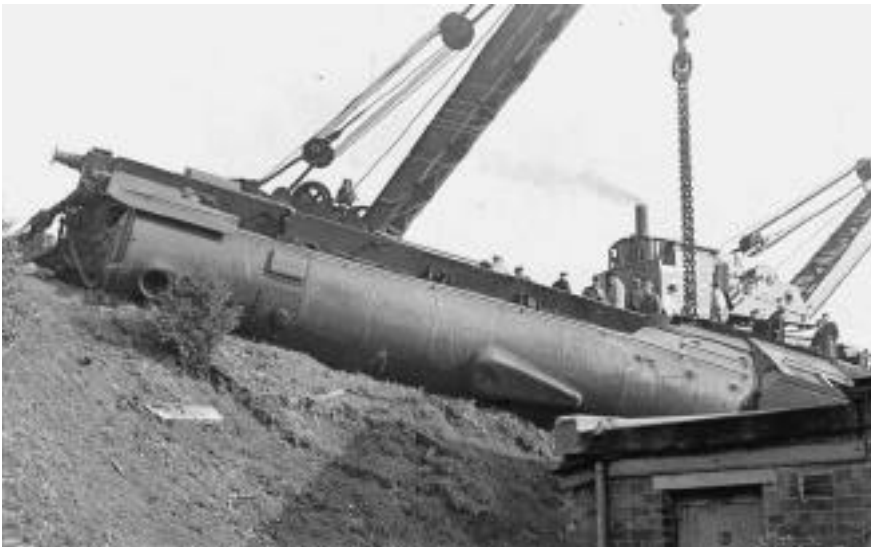
The Peterborough MPD breakdown crane starting to right A1 60123, derailed on the Lincoln avoiding line, October 1949.
