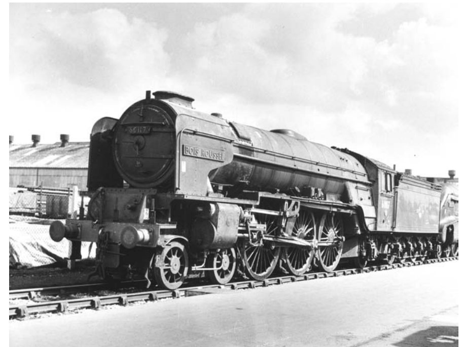
A curiosity: Peppercorn A1 60117 Bois Roussel photographed in Doncaster Works on Sunday 19 May 1963, fitted with an A3 tender of Great Northern pattern. It is not thought to have gone out on the main line in this state: engine (vacuum) and tender (steam) brakes would have been incompatible! (photo: G. W. Morrison)
