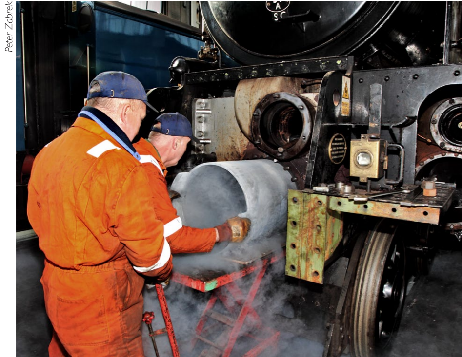
Above: The Bryn Engineering team insert the centre cylinder liner.
