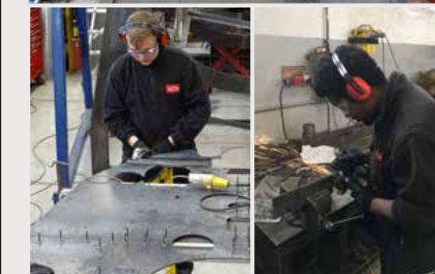
All three apprentices hard at work in the Darlington workshop. Top: David Harrison using mag drill on backhead cladding. Left: James Henshaw angle grinding backhead cladding. Right: Ondre Brooks.
