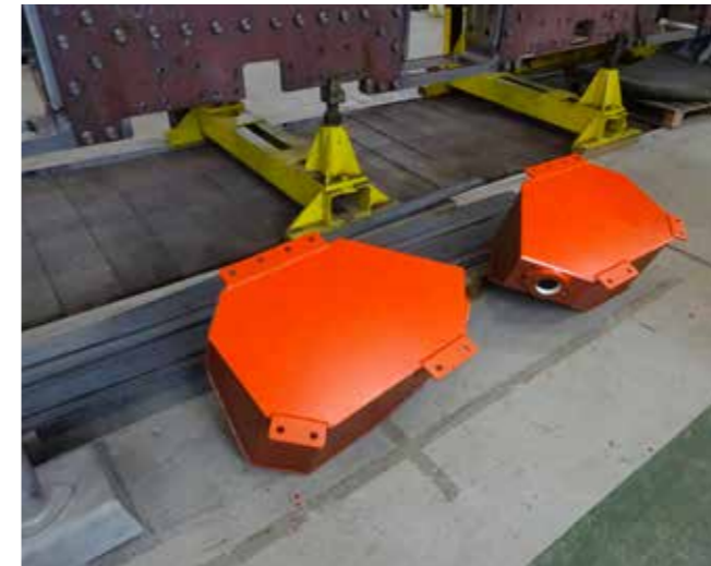
Above: The finished sandboxes painted and ready for final assembly to the frames.
