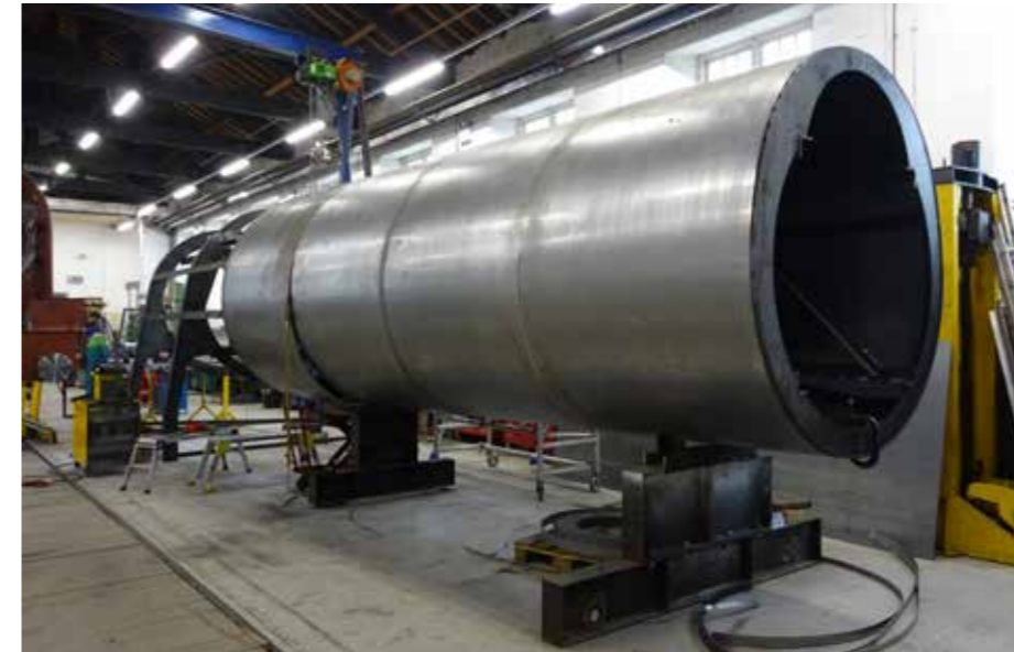
Above: Ian Matthews and the apprentices start to roll the cladding sheets.
