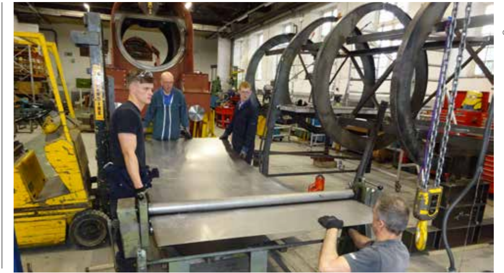
Above: Ian Matthews and the apprentices start to roll the cladding sheets.
