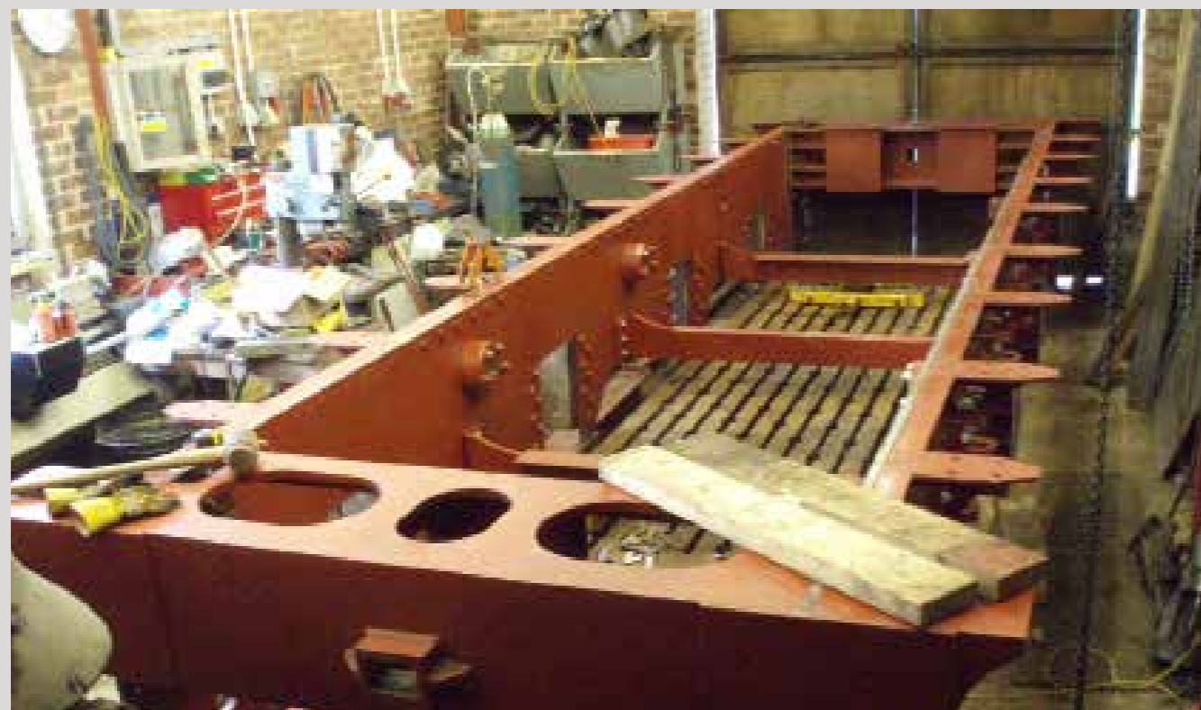
In a process soon to be repeated for No. 2007, Tornado's tender frames are seen under construction at Ian Howitt's engineering works in Crofton.
